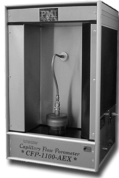
Figure 1. The Microflow Porometer used in this investigation
