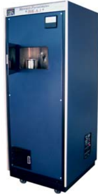
Figure 2. The Mercury Intrusion Porosimeter used in this investigation
