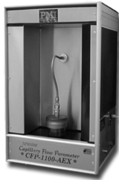
Figure 4. The PMI capillary flow porometer with capability to measure gas and liquid flow rates.
