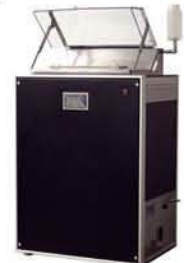
Figure 3. Liquid Permeameter used in this study
